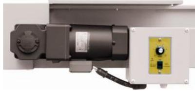
Picture 6-1: Gear motor
